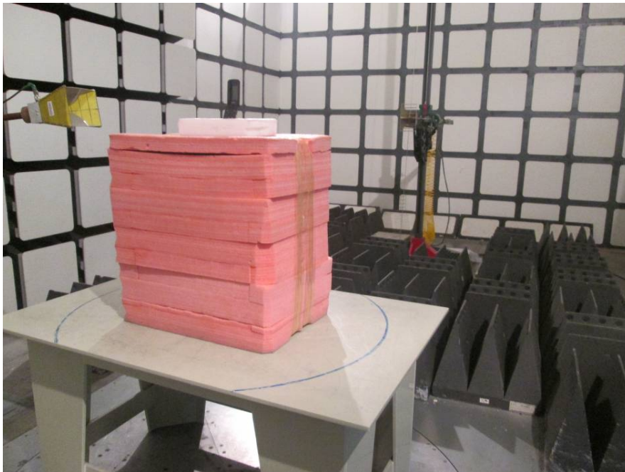
Radiated Emissions Test View (Above 1 GHz)
