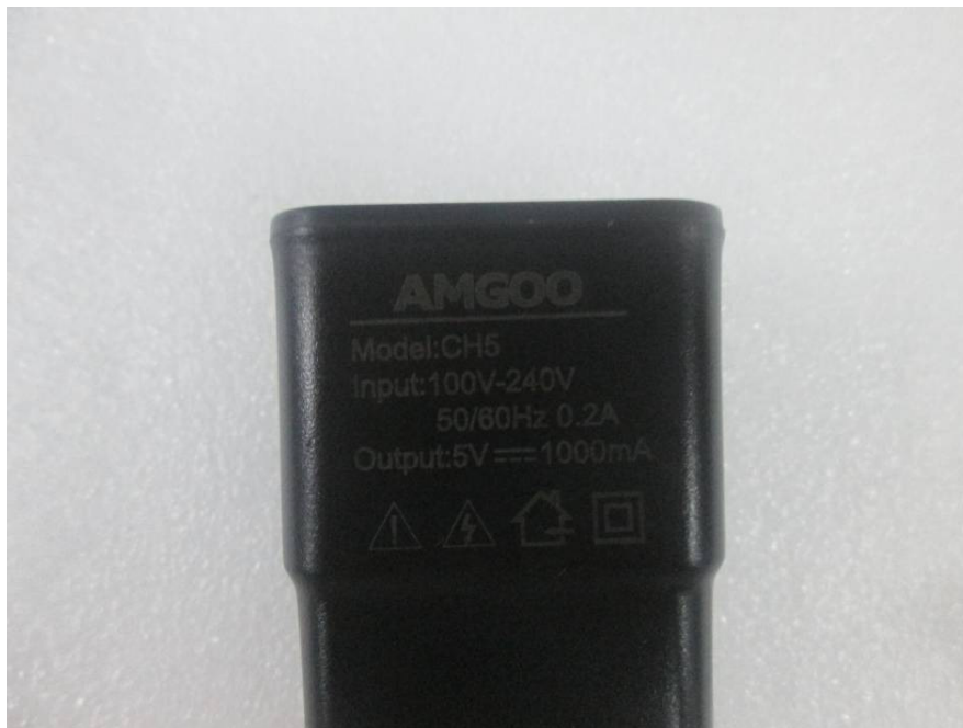
EUT – Adapter Label View
