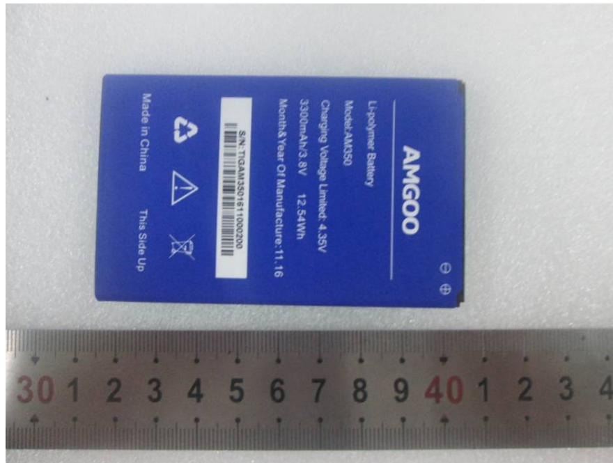
EUT – Battery Front View
