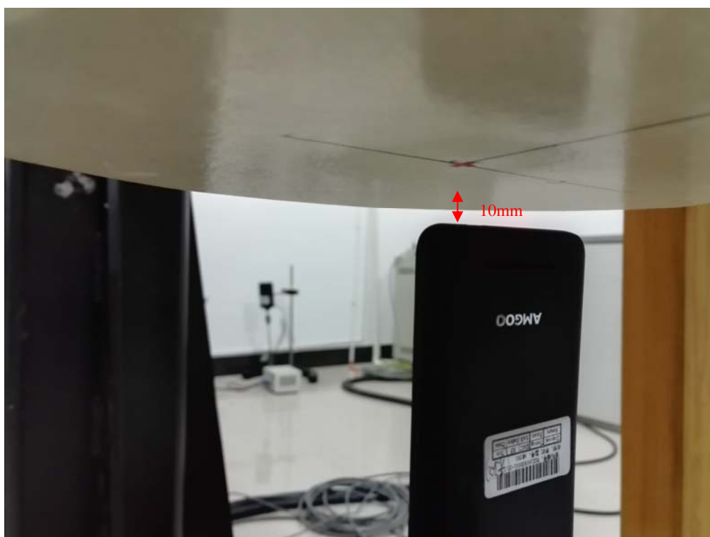
Body-worn Bottom Setup Photo (10mm)
