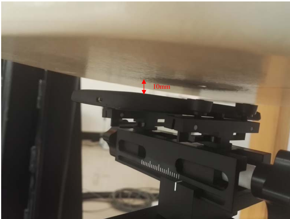
Body-worn Back Setup Photo (10mm)
