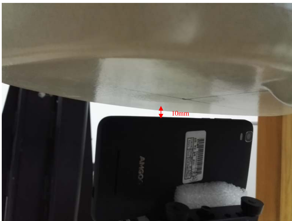
Body-worn Right Setup Photo (10mm)
