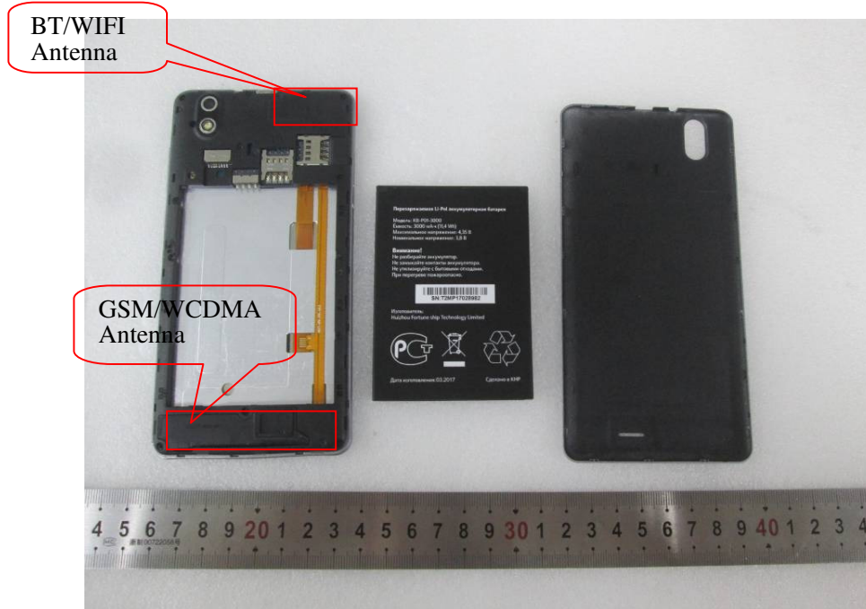
EUT – Cover off View 1
