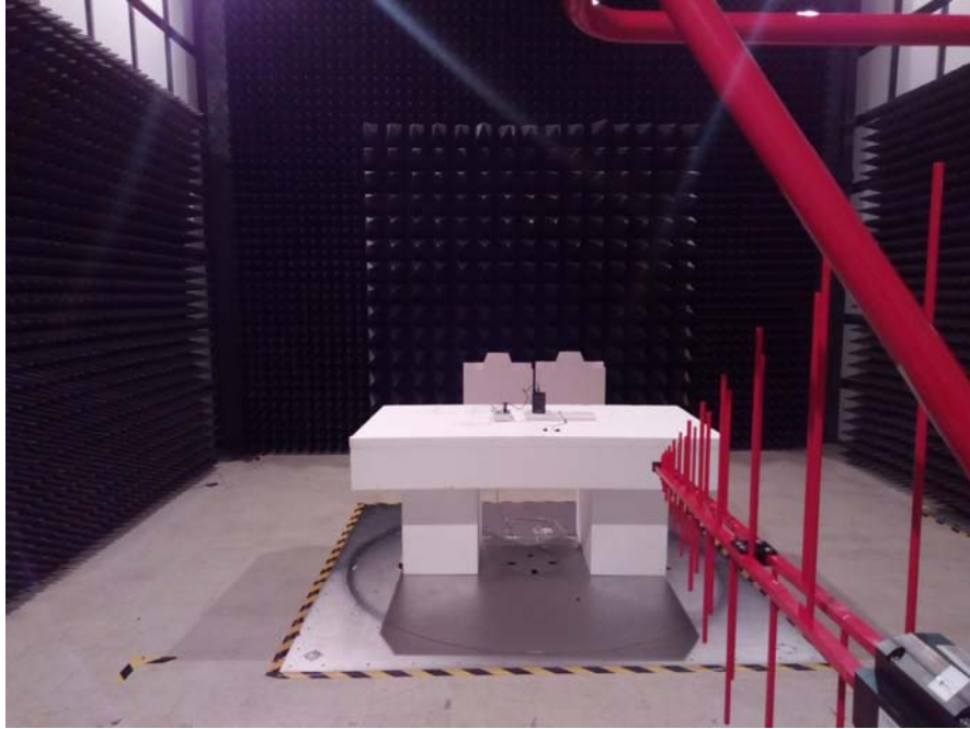
Radiated Emissions View (Below 1 GHz)
