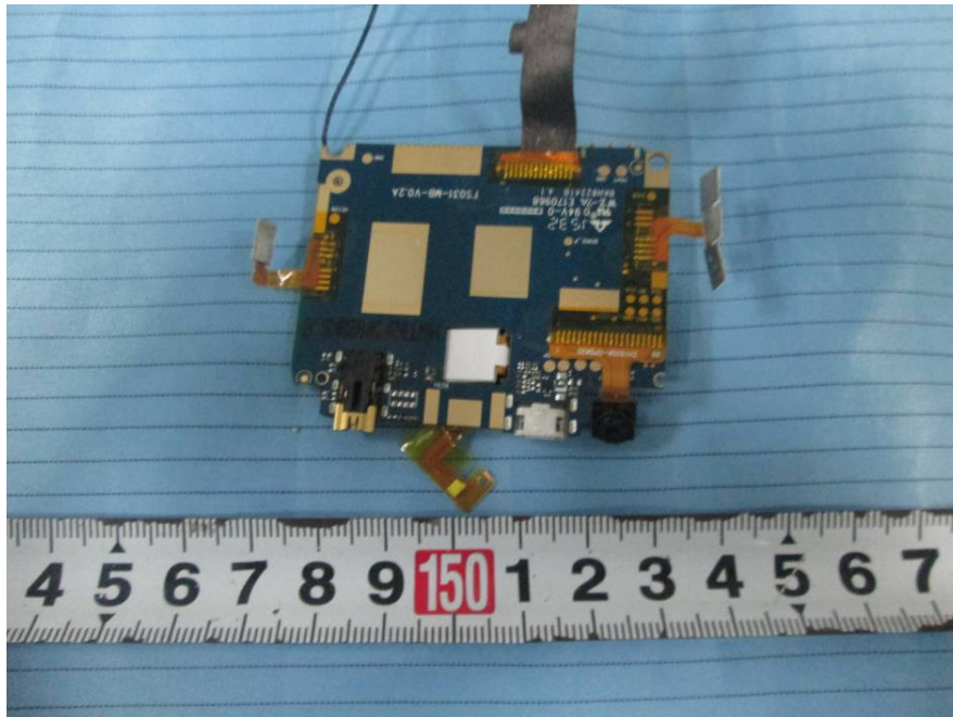
EUT – Main Board 2 Top Shielding off View
