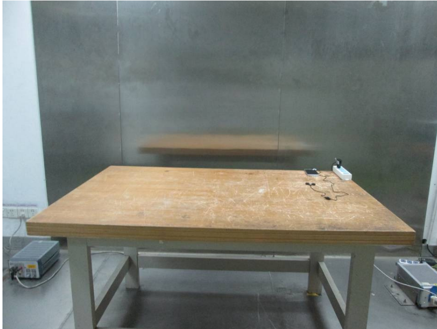
Conducted Emissions - Front View
