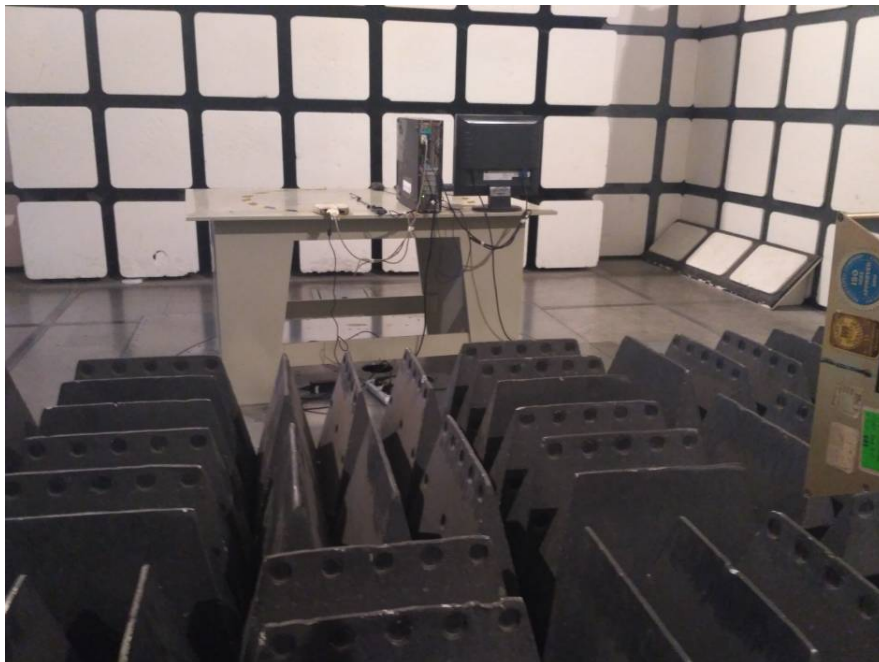
Radiated Emissions – Rear View (Above 1 GHz)
