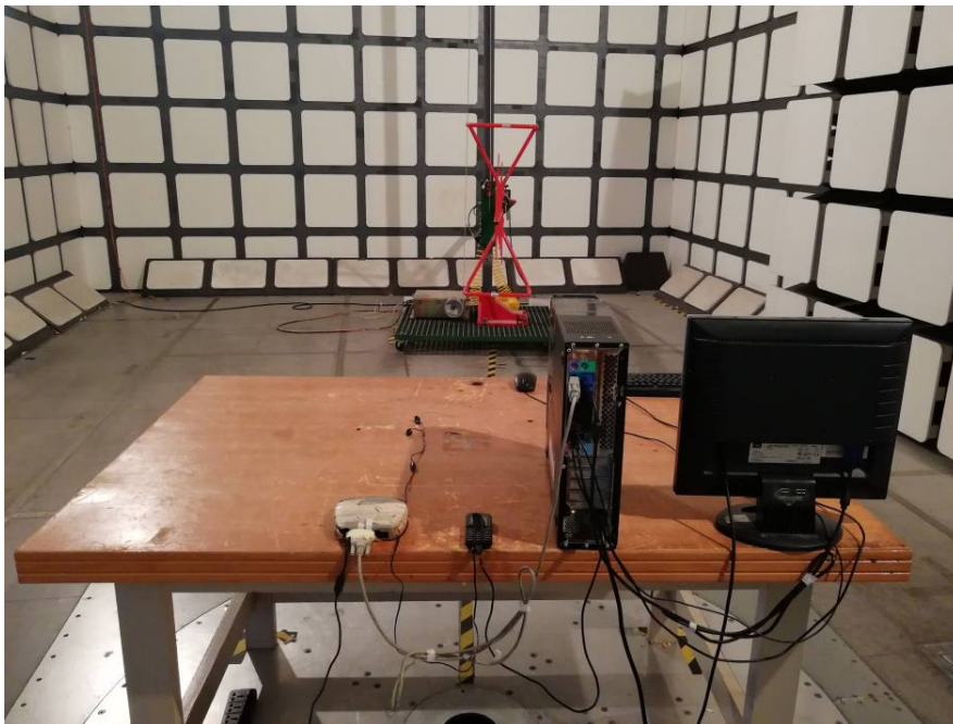
Radiated Emissions – Rear View (Below 1 GHz)
