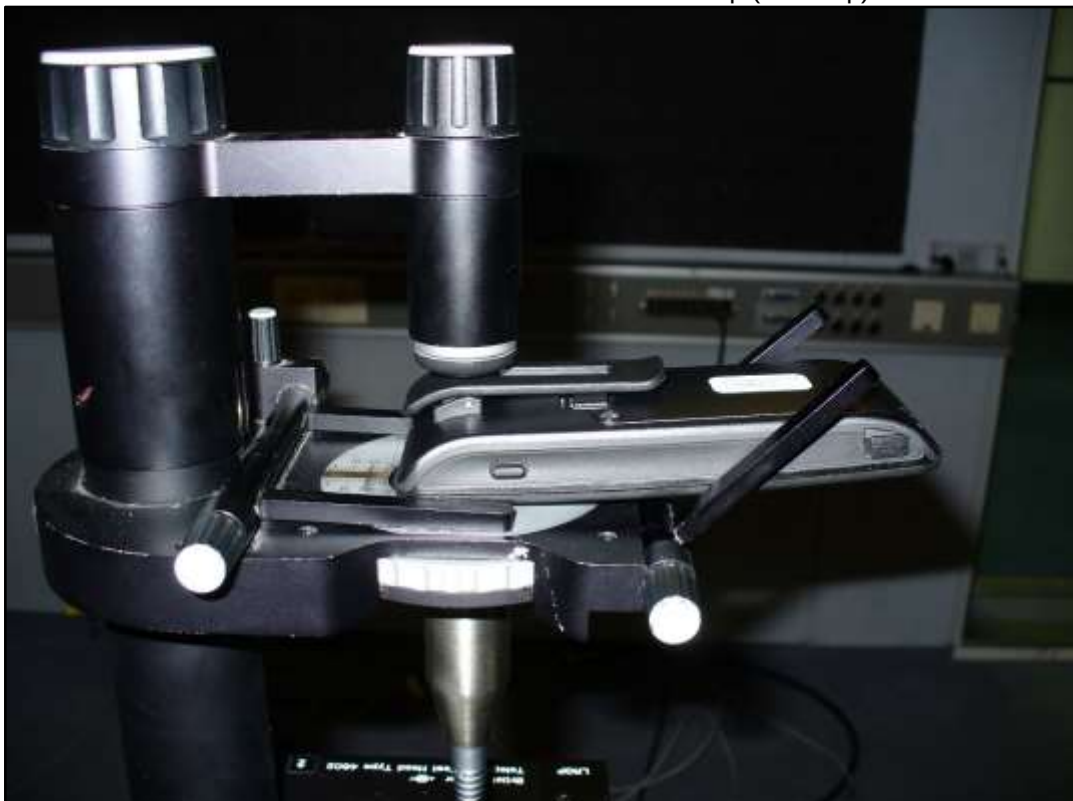
Photo 2: Volume control measurement set-up (close-up)
