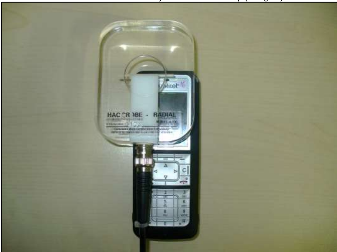
Photo 4: Radial field intensity measurement set-up (0 degree)
