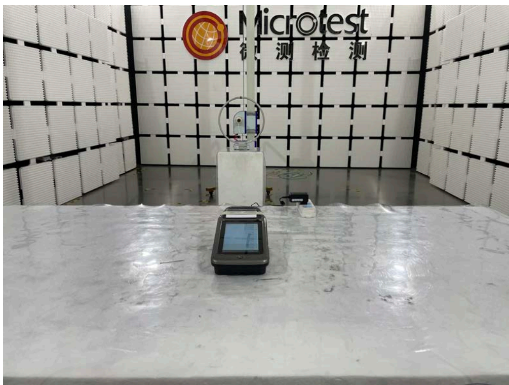
Radiated emission – below 1GHz
