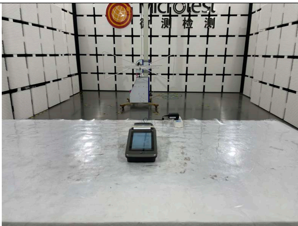
Radiated emission – below 1GHz
