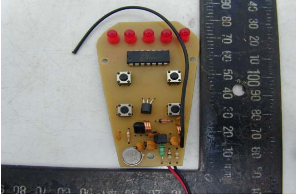
Component Side of Main Board of Remote Controller
