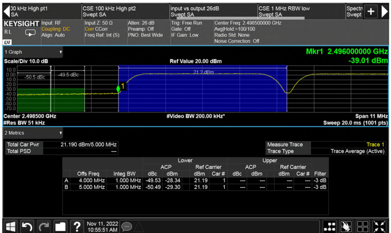
Plot of lower band edge for Low channels (2498.5 & 2503.5MHz)
