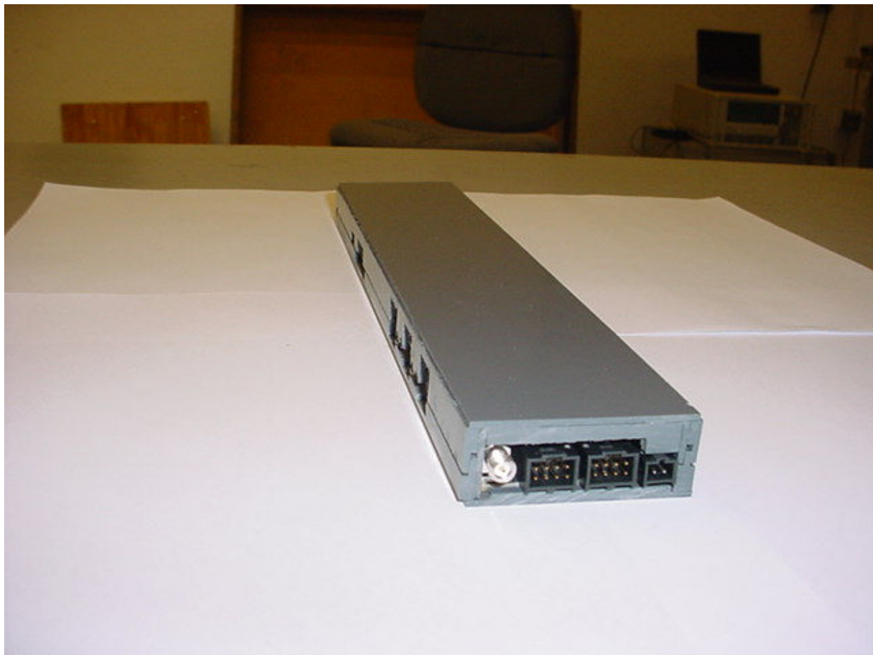
Side View (antenna, power, magnetic switches connectors)
