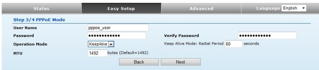
The screenshot shows the 'Easy Setup' menu with 'Step 3/4 PPPoE Mode' selected. The form contains the following fields: User Name (pppoe\_user), Password (masked with dots), Verify Password (masked with dots), Operation Mode (KeepAlive), and MTU (1492 bytes). There are 'Back' and 'Next' buttons at the bottom.
