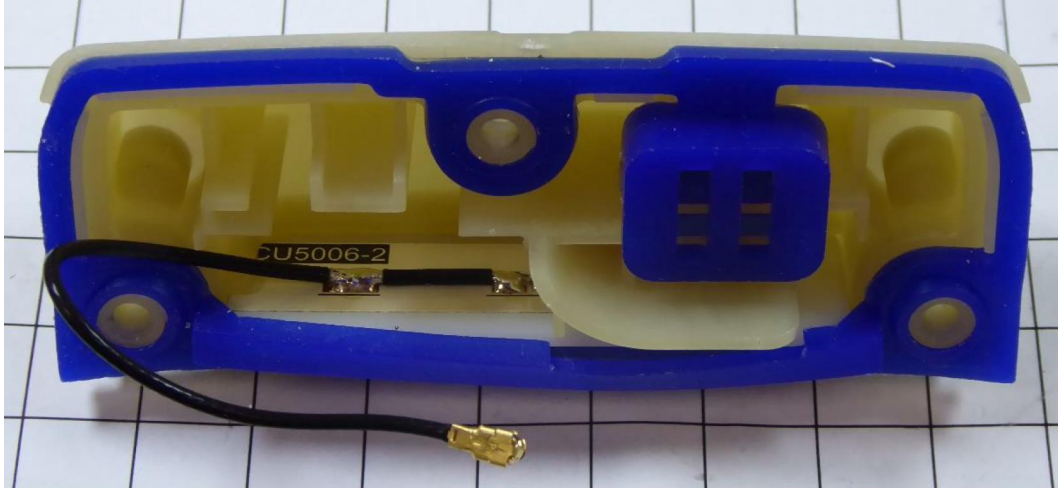
WCM 9116 with attached wires to access test modes:
