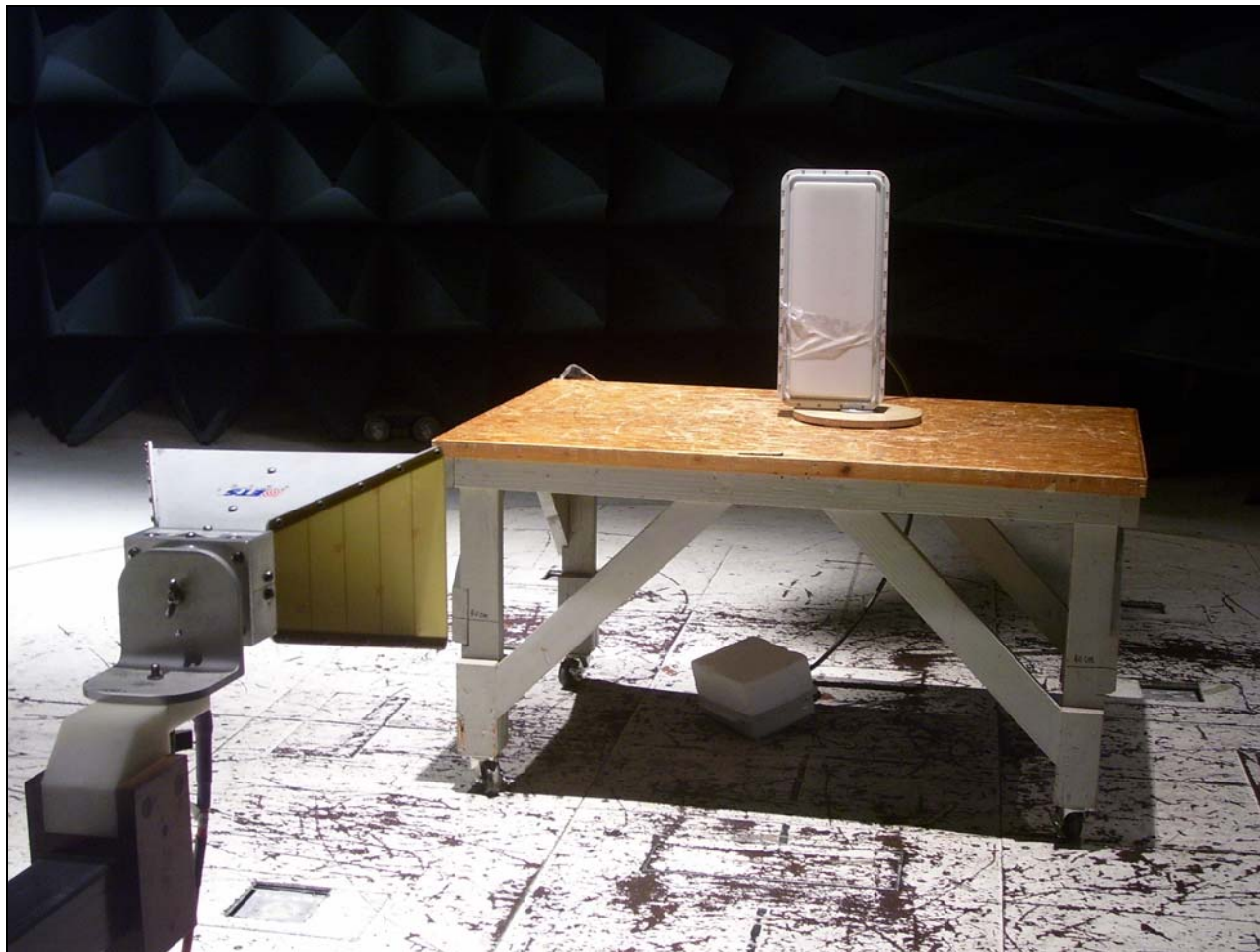
Photograph 14. Test Equipment and setup for various Radiated Measurements, MT-484034-NV Antenna
