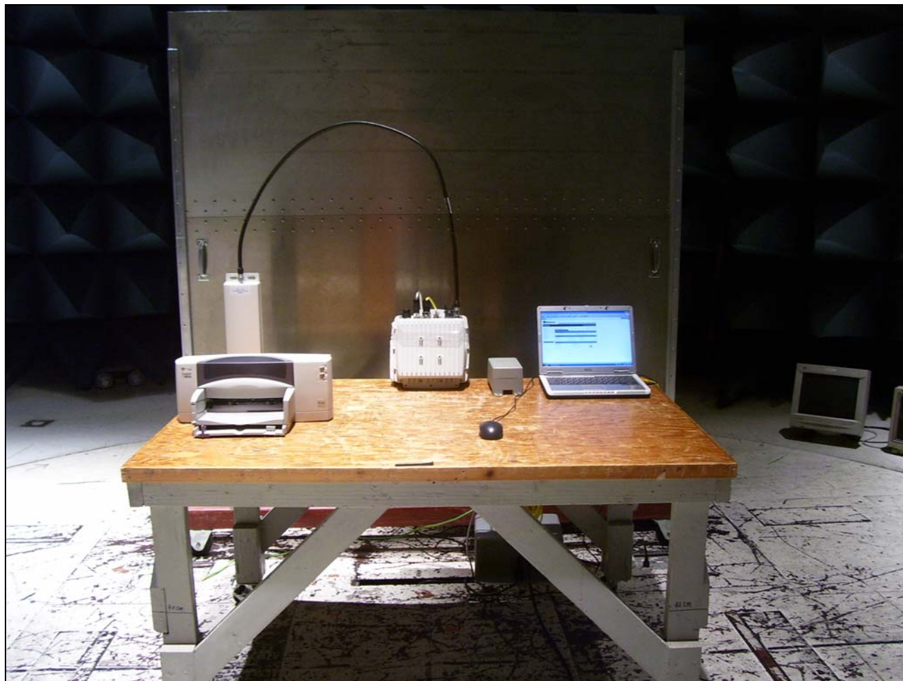
Photograph 4. Conducted Emissions Test Setup for ASN-800FCC-N
