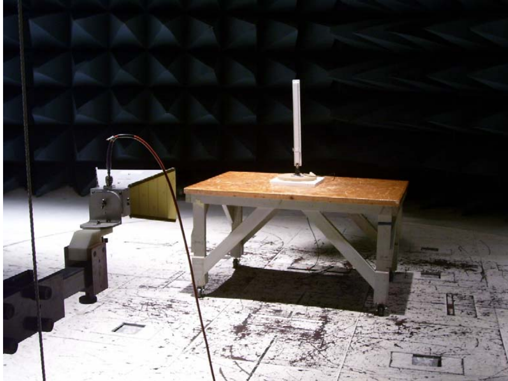
Photograph 6. Test Equipment and setup for various Radiated Measurements
