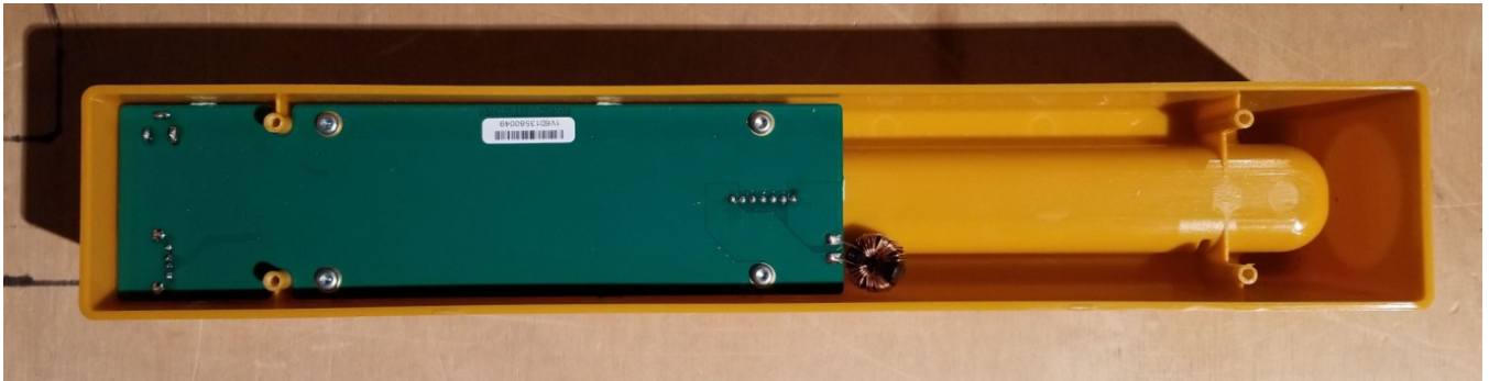
Photograph 25 - USB docking cradle bottom view with bottom removed
