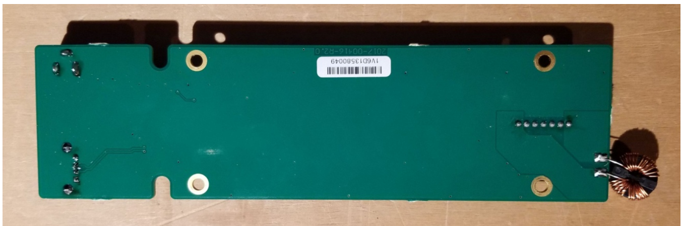
Photograph 27 - 2400-00427-R2 USB docking cradle circuit board top side
