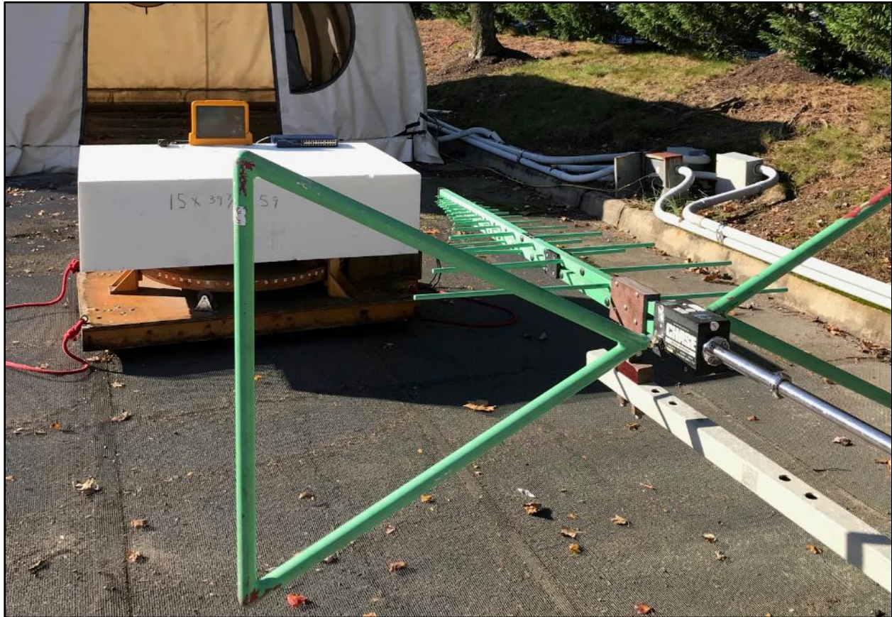
Photograph 2: Radiated Emissions Testing: Below 1 GHz – Front View
