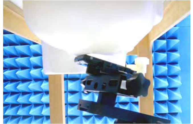
Figure 14. Right Head SAR Test Setup (Tilted)
