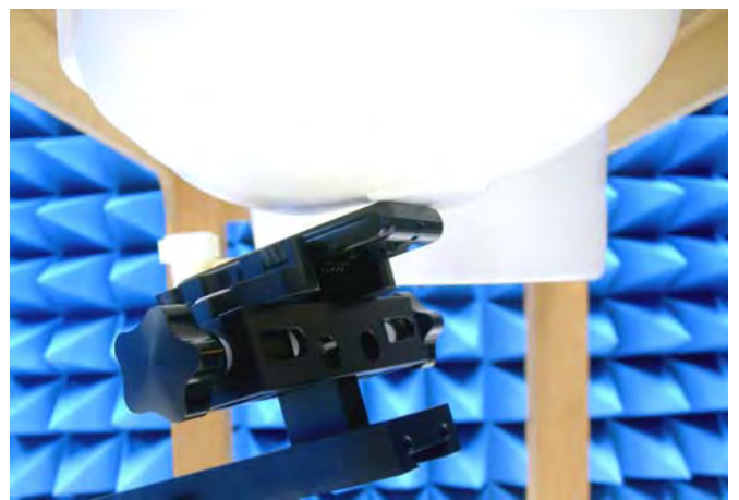
Figure 16. Left Head SAR Test Setup (Tilted)
