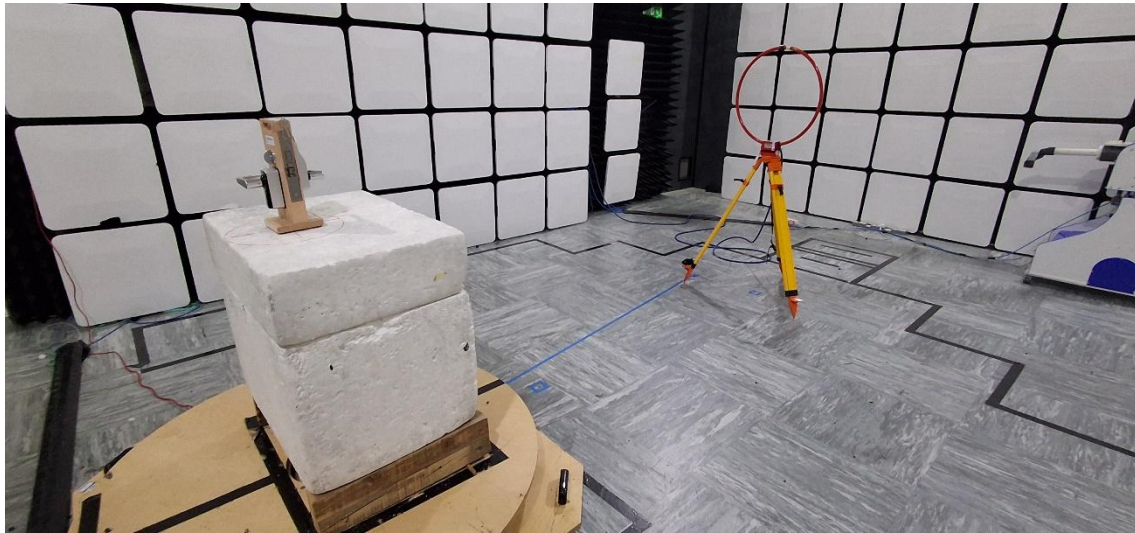
Figure 10 - Test Setup – 9kHz to 30MHz Front-On
