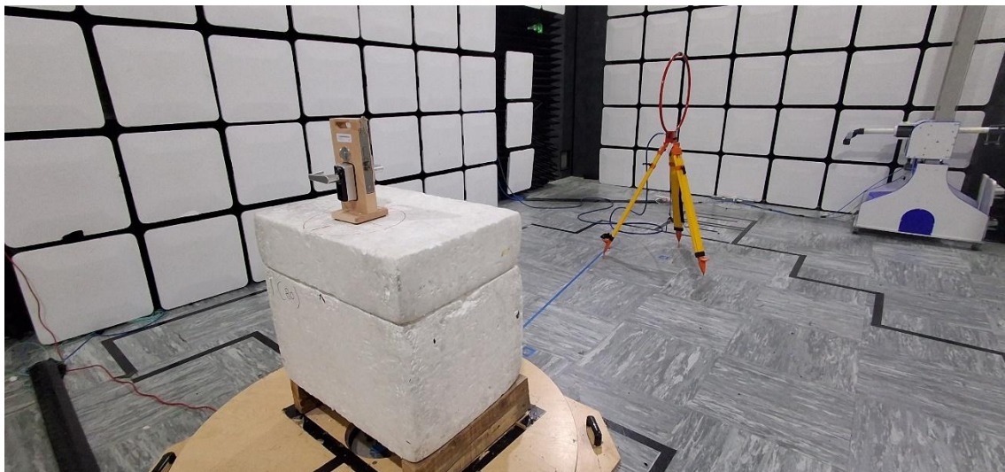
Figure 11 - Test Setup - 9kHz to 30MHz Side-On
