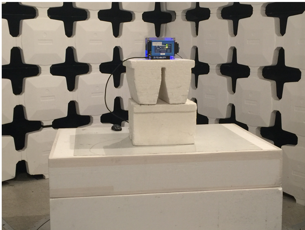
Figure 1. Radiated Emissions Test Setup, Close-up
