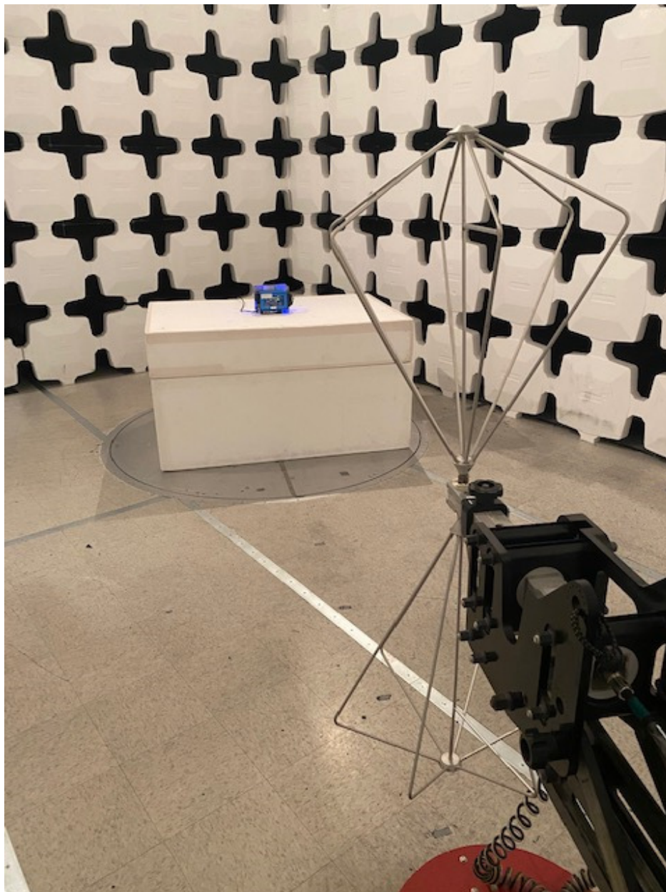
Figure 3. Radiated Emissions Test Setup, 30 MHz to 200 MHz
