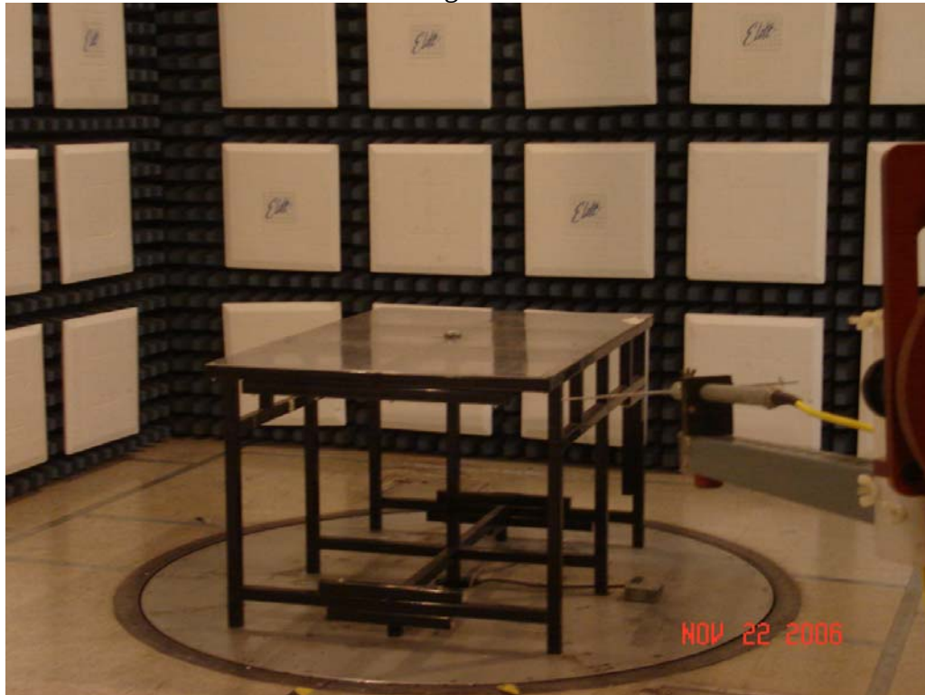
Test Setup for Radiated Emissions, 433.9MHz – Horizontal Polarization
