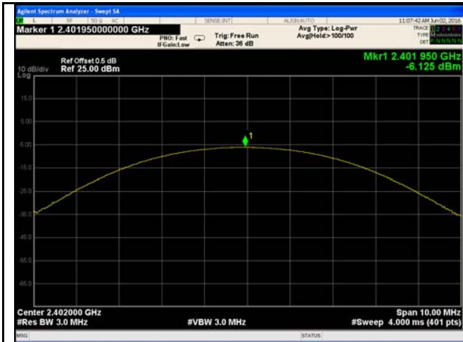
8DPSK Output power - Low CH 2402
