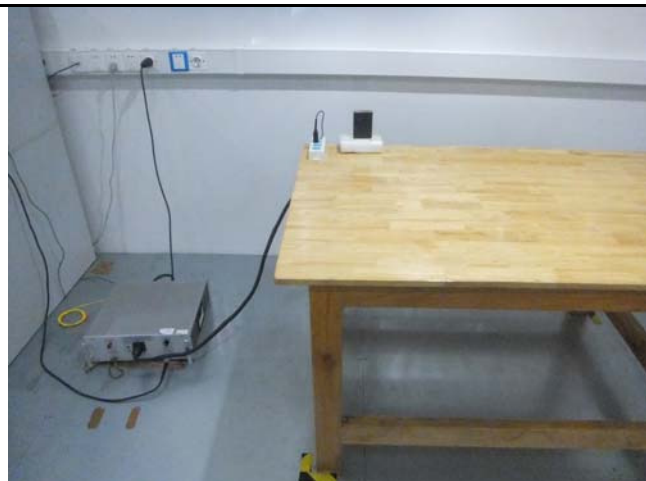
Conducted Emissions Test Setup Front View
