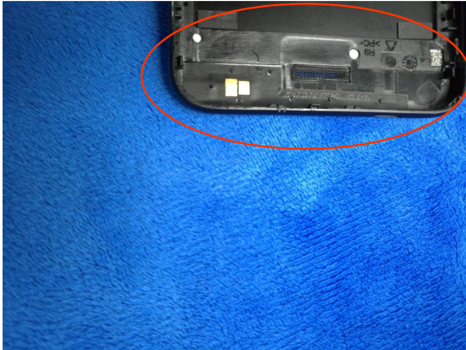
GSM/PCS/UMTS - Antenna View
