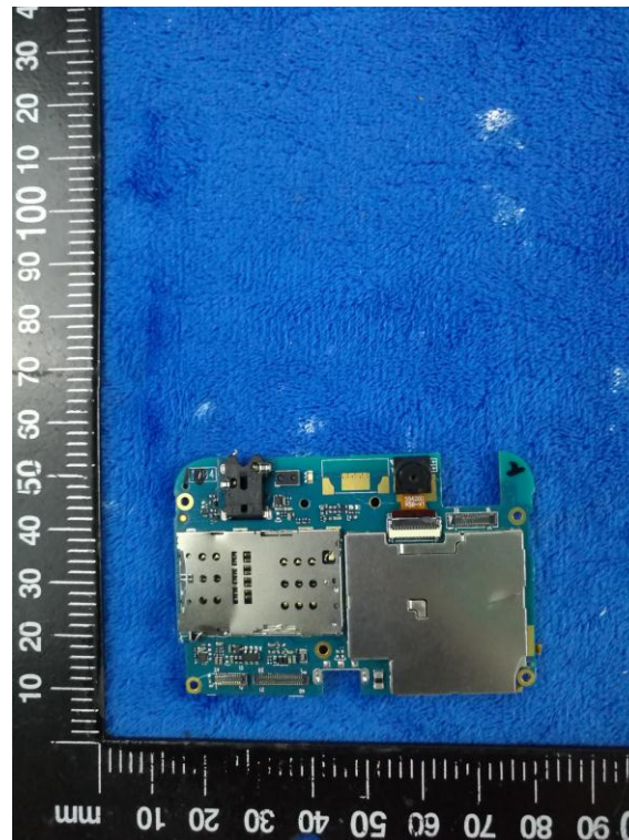
Mainboard with Shielding - Rear View
