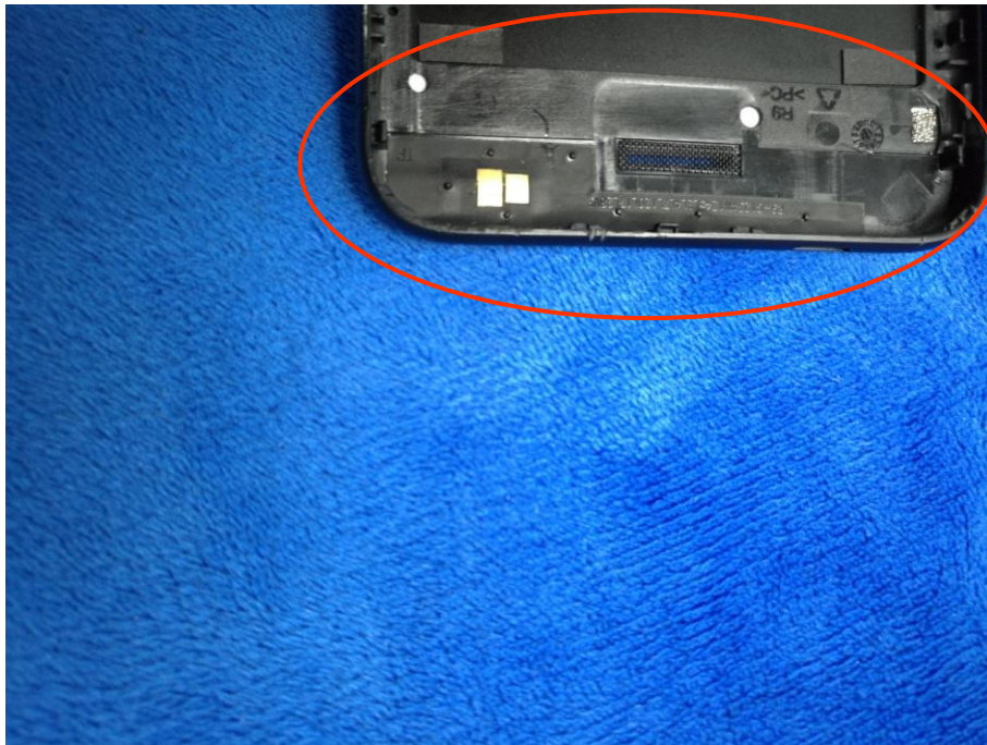
GSM/PCS/UMTS - Antenna View
