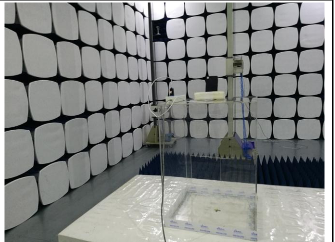
Radiated Spurious Emissions Test Setup Above 1GHz
