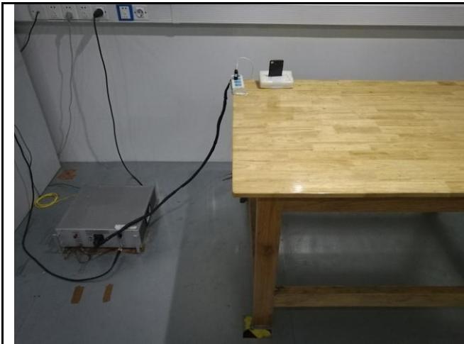
Conducted Emissions Test Setup Front View
