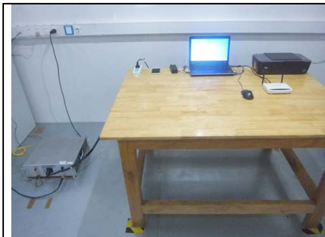
Conducted Emissions Test Setup – Front View
