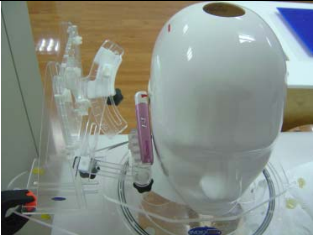
Fig.5 EUT Right Head Touch Cheek Position
