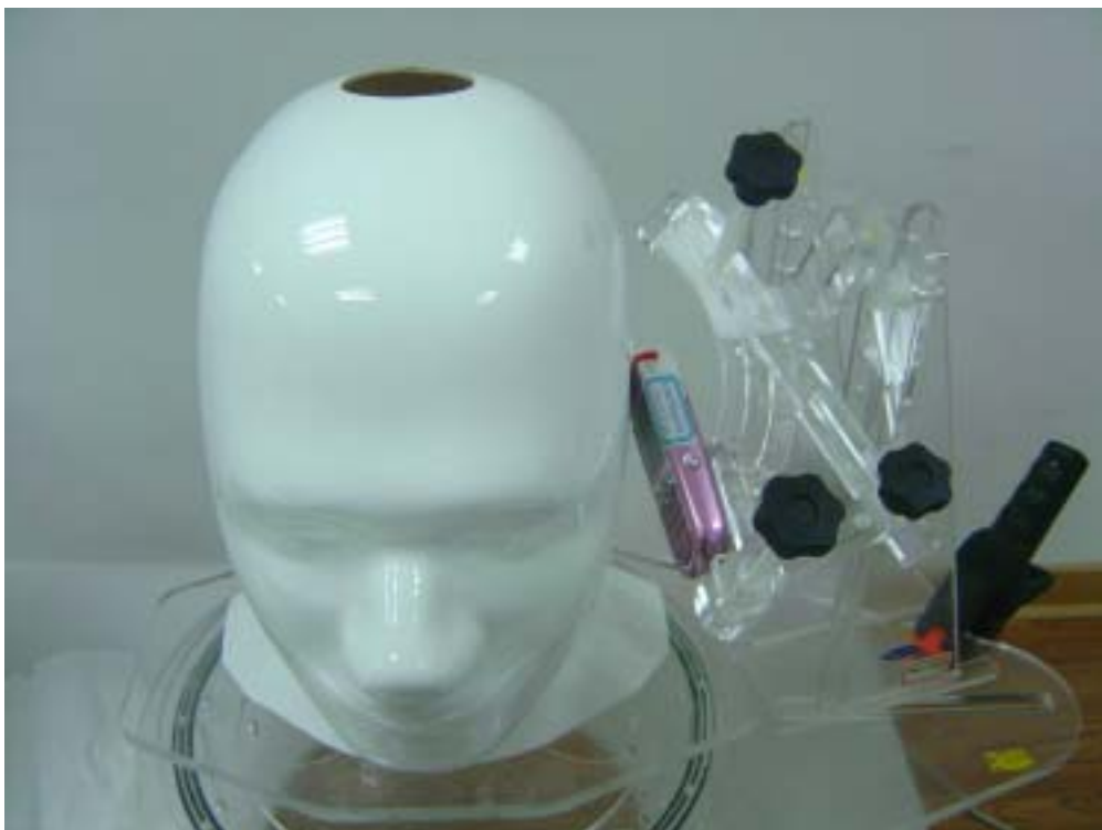
Fig.4 EUT Left Head Tilt15 Position
