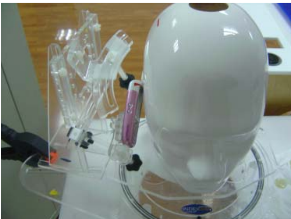
Fig.6 EUT Right Head Tilt15 Position
