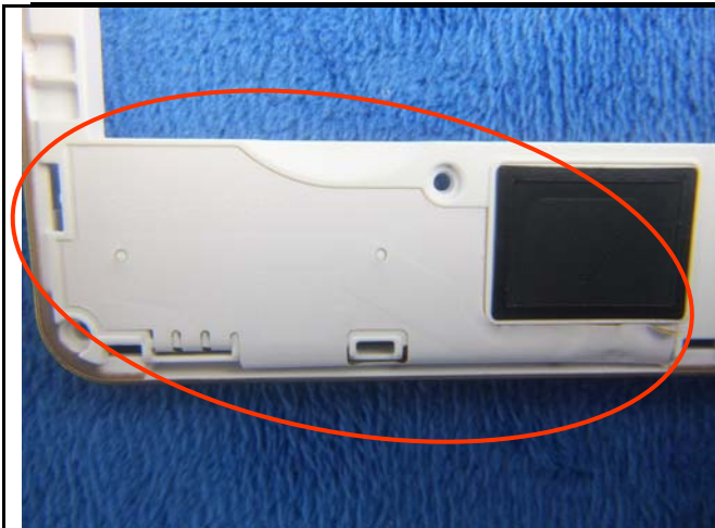
GSM/PCS/UMTS-FDD Antenna View
