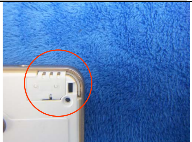
WIFI/BT/BLE/GPS - Antenna View
