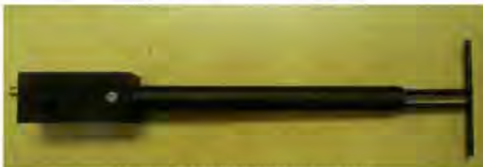
Figure 1 – MVG COMOSAR Validation Dipole
