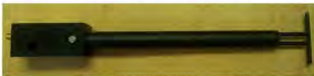
Figure 1 – MVG COMOSAR Validation Dipole
