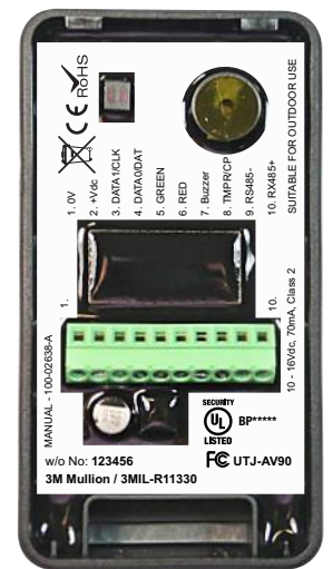
VIEW - REVERSE ▲ internal view assembled and POTTED
