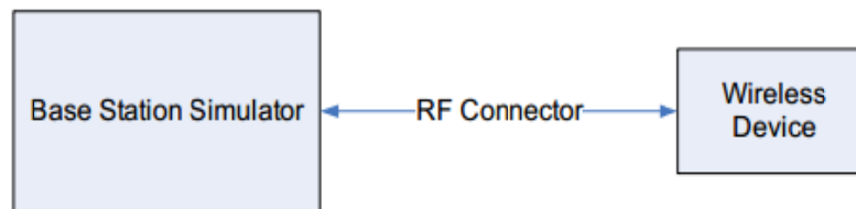
Figure 10.2 Power Measurement Setup
