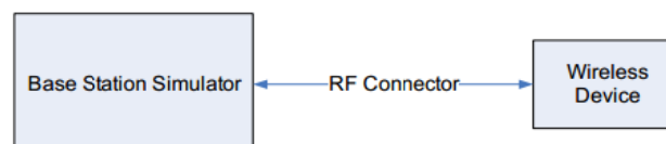
Figure 10.1 Power Measurement Setup
