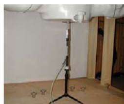
Figure 11.1 Dipole Verification Test Setup Diagram & Photo
