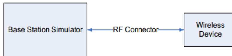
Figure 10.2 Power Measurement Setup
