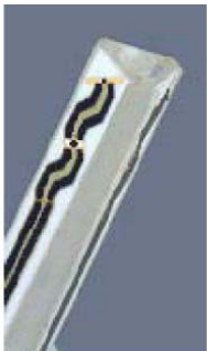
Figure 3.3 Probe Thick-Film Technique
