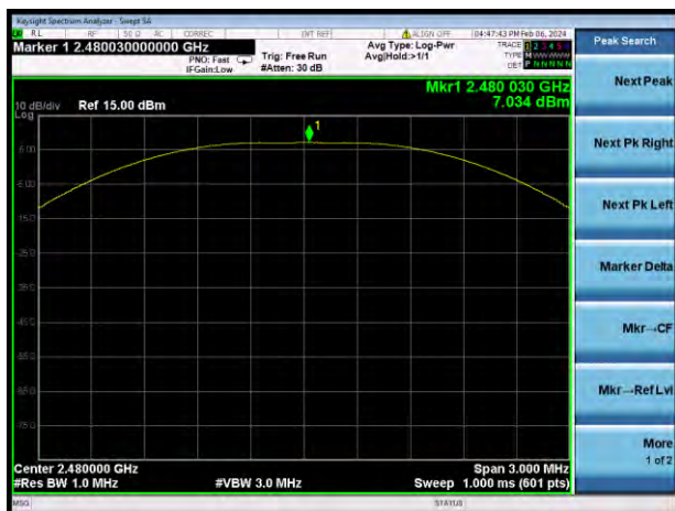
GFSK (BLE 1Mbps) HIGH CHANNEL
