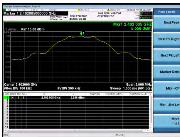
GFSK (BLE 1Mbps) LOW CHANNEL, CARRIER LEVEL
