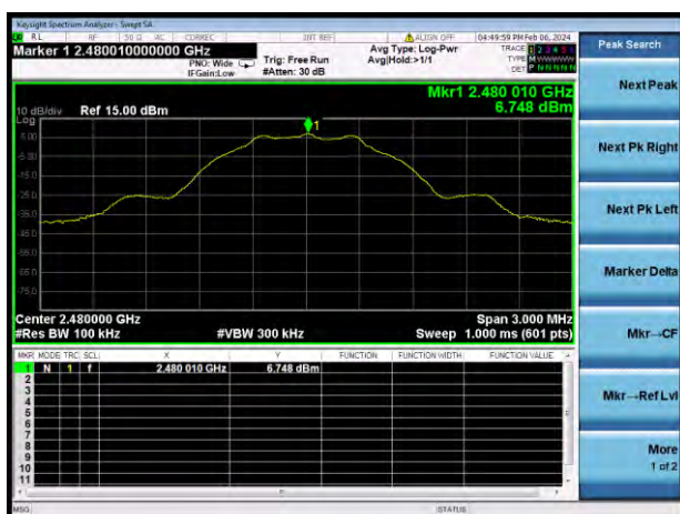
GFSK (BLE 1Mbps) HIGH CHANNEL, CARRIER LEVEL
