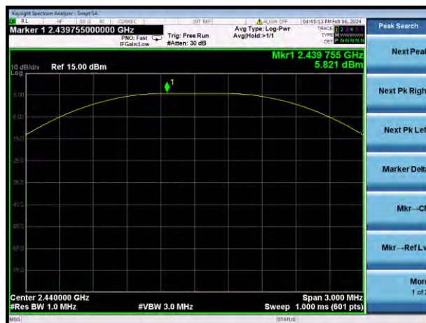
GFSK (BLE 1Mbps) MIDDLE CHANNEL
