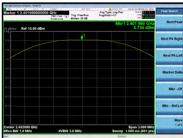
GFSK (BLE 1Mbps) LOW CHANNEL
