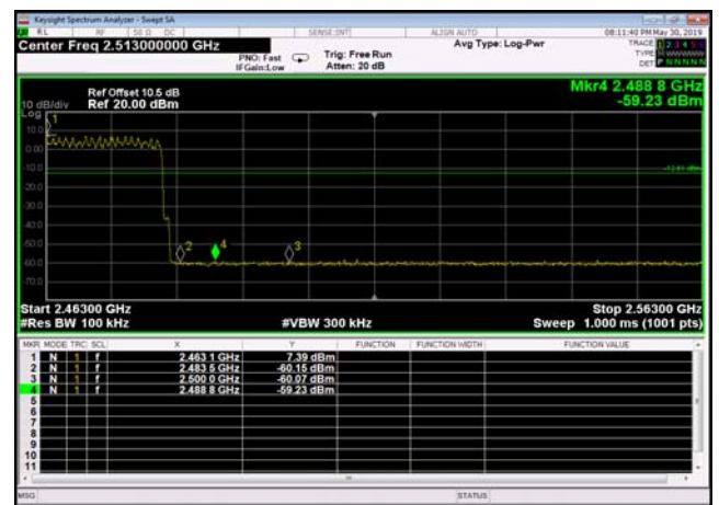
Conducted Emission: 8DPSK,2480,3DH5 ,Band Edge
