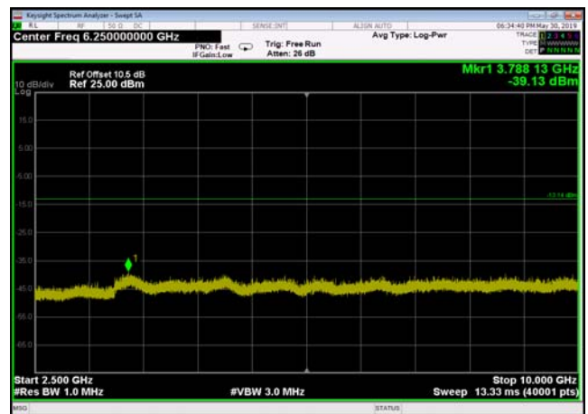
Conducted Emission: GFSK,2480,DH5 ,2500MHz~10000MHz
