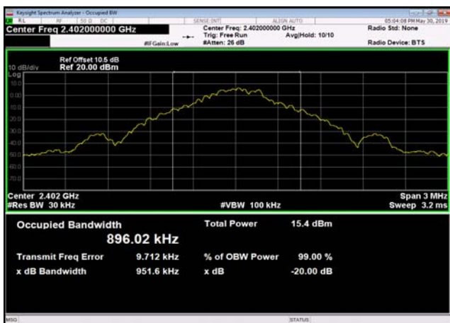
99% Bandwidth: GFSK,2402MHz,DH5
