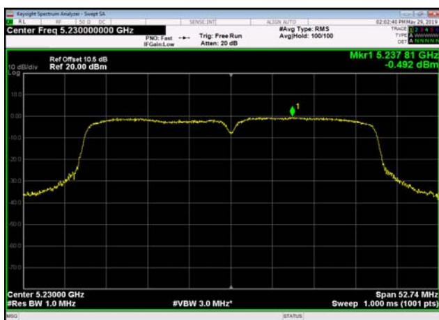
U-NII-1 Power spectral density-802.11 n(40MHz),5230MHz
