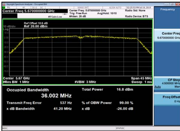
U-NII-2c 99% Bandwidth-802.11ac(80MHz) ,5610MHz
