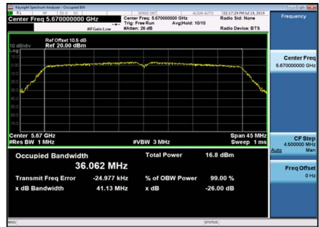
U-NII-2c 99% Bandwidth-802.11a(20MHz) ,5600MHz
