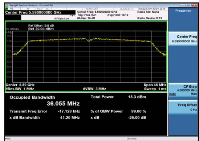
U-NII-2c 99% Bandwidth-802.11ac(80MHz) ,5530MHz
