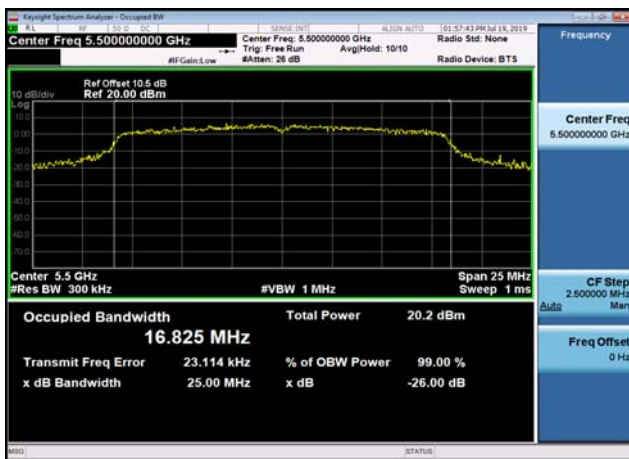
U-NII-2c 99% Bandwidth-802.11a(20MHz) ,5700MHz
