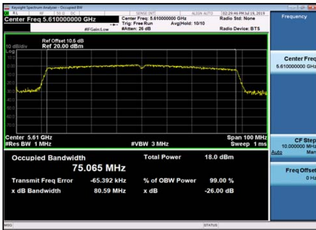
U-NII-2c 99% Bandwidth-802.11ac(80MHz) ,5610MHz
