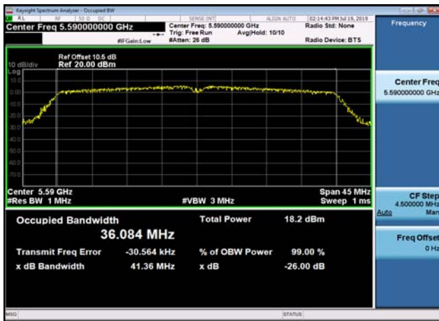
U-NII-2c 99% Bandwidth-802.11a(20MHz) ,5500MHz
