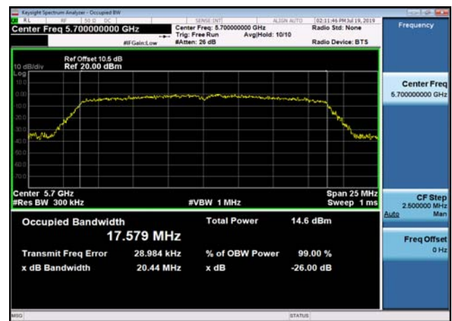
U-NII-2c 99% Bandwidth-802.11ac(40MHz) ,5590MHz
