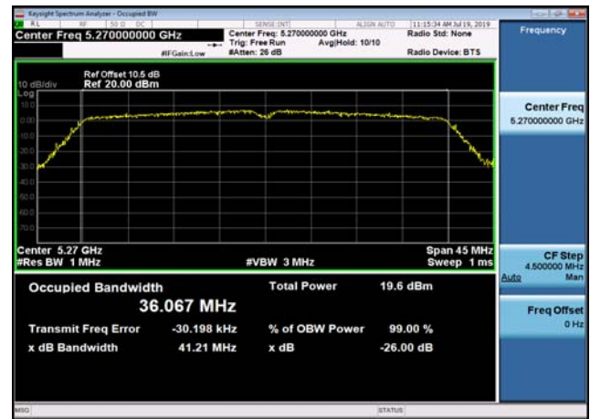
U-NII-2a 99% Bandwidth-802.11ac(80MHz) ,5290MHz
