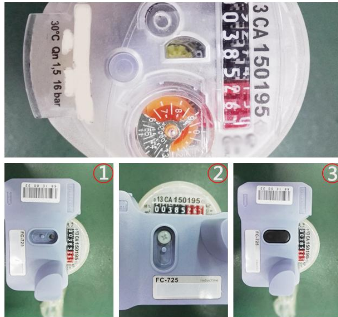
Figure 5-2 Installation of IDUV915-LRW
