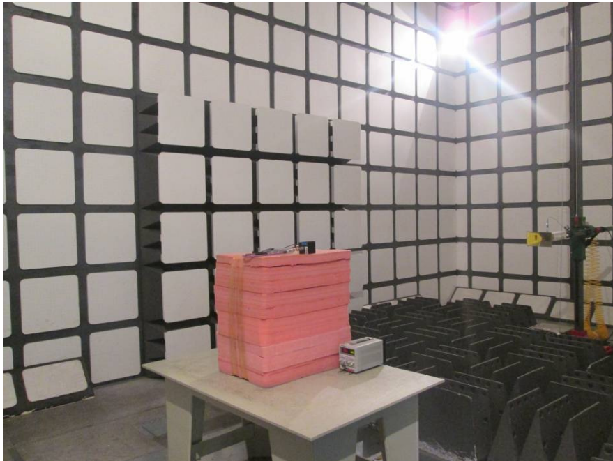
Radiated Emissions – Front View (Above 1 GHz)
