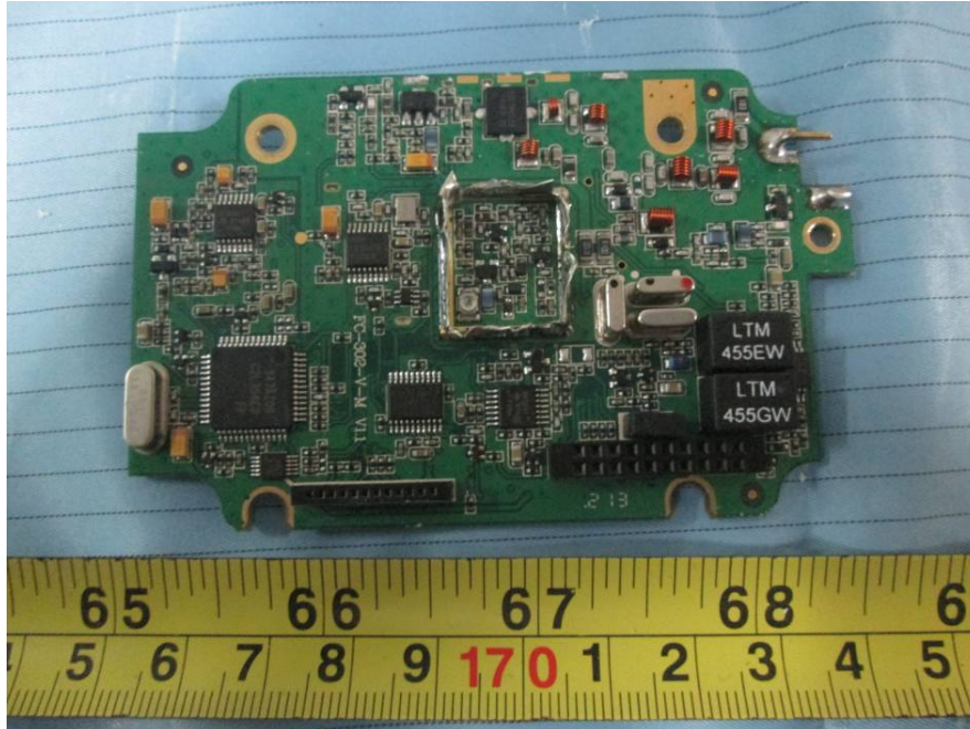
EUT –Main Board Top Shielding Off View
