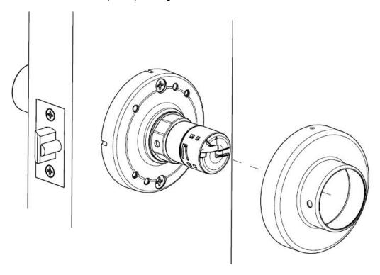
B. Install the inside lever handle. Fasten inside lever handle with setscrew inserted in the side hole of the inside rose.
