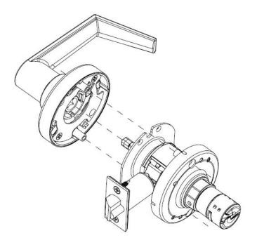
B. With the battery arrow pointing up on the inside, slide the outside lever assembly onto the lock shaft. Fasten rose assembly with two through bolts from the inside.
