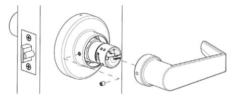
Twist the inner rose so that the access hole is aligned with the latch and exposing the set-screw.
