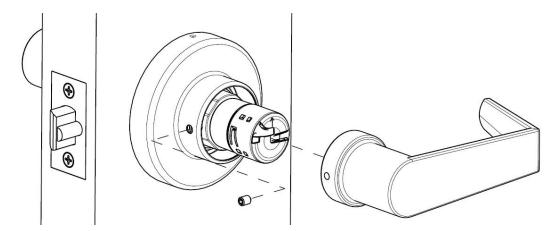
**C.** Rotate the rose so that the side hole faces down. The rose will snap in to place.
