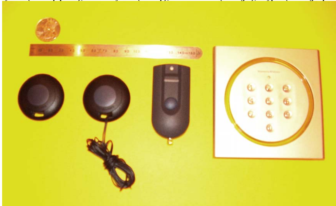
Simons-Voss Entry Transponders: Key-Fob (Far Left photo), Wired Key Fob (2 nd Left), Biometric Fob(2 nd Right), Keypad (Far Right photo)
