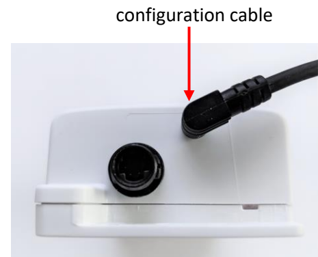
7-5-1 VP Essentials Sensor Top Side View Showing Configuration Port and Cable
