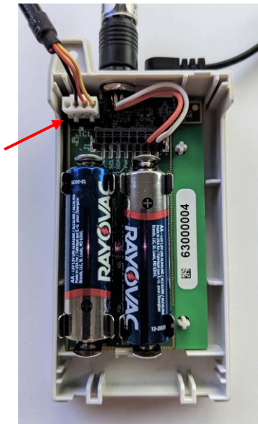
7-5-2 VP Essentials Sensor Top Side View Showing Configuration Port and Cable
