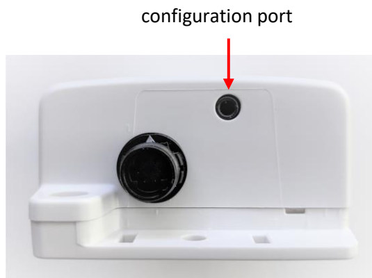
7-5-1 VP Essentials Sensor Top Side View Showing Configuration Port and Cable
