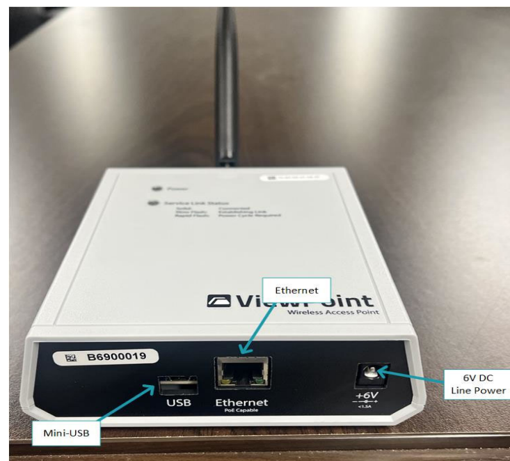
Fig. 3.1-2 – Access Point 1.1 Equipment Details
