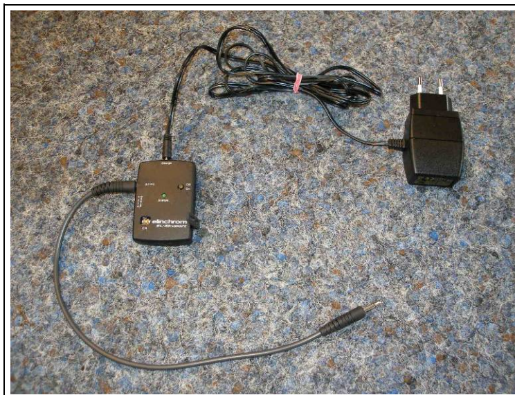
EL-Skyport Universal Receiver with synchron cable and external AC/DC power supply
