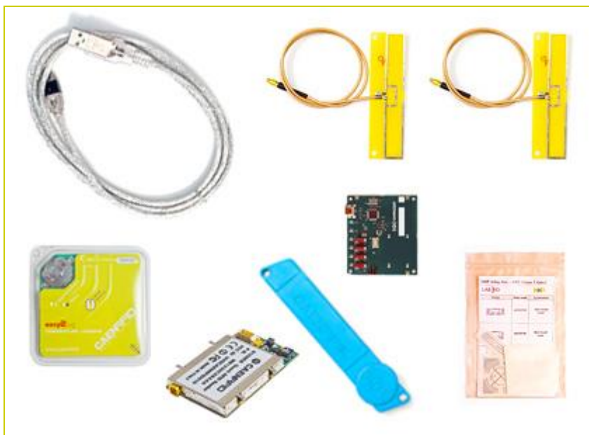
Fig. 1.4: R1230DK quark Ultra Compact Embedded UHF RFID Reader Development Kit
