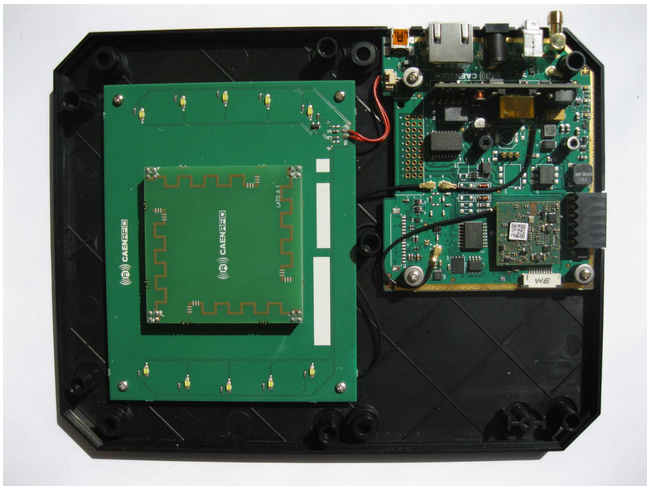
Figure 3 - Host board with RF switch
